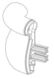
2. Attach Returns and Corners to retainer, leaving 1/16" [2mm] gap between Return/Corner and retainer allowing for adjustment. **See Fig. 3**.
