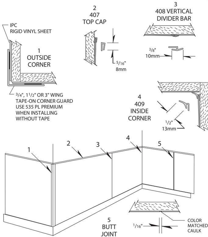
FOR .080" THICK SHEET, USE 417 TOP CAP, 418 VERTICAL DIVIDER BAR AND 419 INSIDE CORNER
